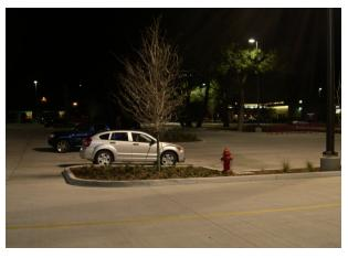
Further calculations showed that comparable luminance could also be achieved on the concrete parking lot with a reduction in illuminance. In fact, if the wattage in each of the 22 luminaires on the concrete lot was reduced from 400 W to 250 W, the average luminance of .336 cd/ft² was still greater
