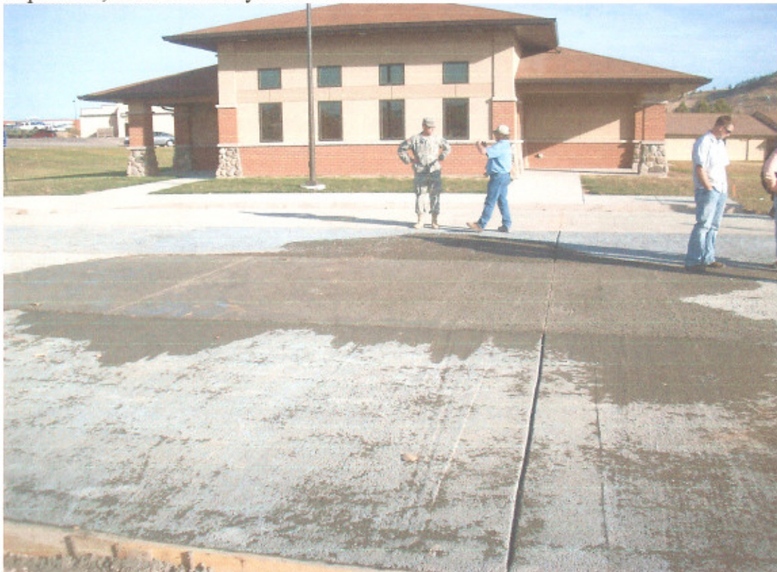
Figure 1 800 gallons of water soaked through 100 square feet of this pervious concrete parking lot in 2 minutes.
